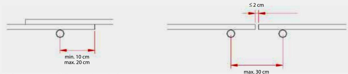
Figure 5.6: Arrangement of the wooden planks
