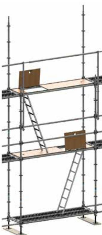
Figure 8.19: Fitted mounting safety guardrail (MSG)
